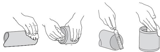
4 Apply cleaner solution to the outside surface of the pipe and to the inside surface of the fitting. Cleaner will prepare the surface for jointing for a better quality joint.
