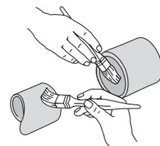
6 While both surfaces are still wet with solvent cement, insert the pipe into the fitting in a single movement. Do not stop halfway, since the bond will start to set immediately and it will be almost impossible to insert further. For a better distribution of the solvent cement, twist the pipe a 1/4 turn during insertion into the socket.
